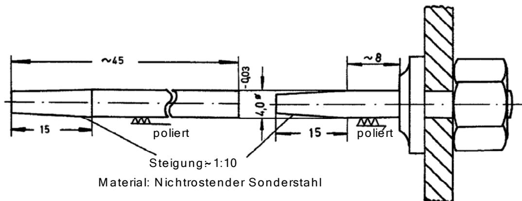
The preferred material for the pin is stainless steel (e.g. X 12 Cr Si 17).
