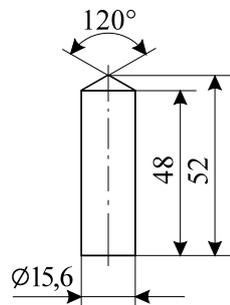
Fig. 2: Cylindrical bronze piston; dimensions in mm
