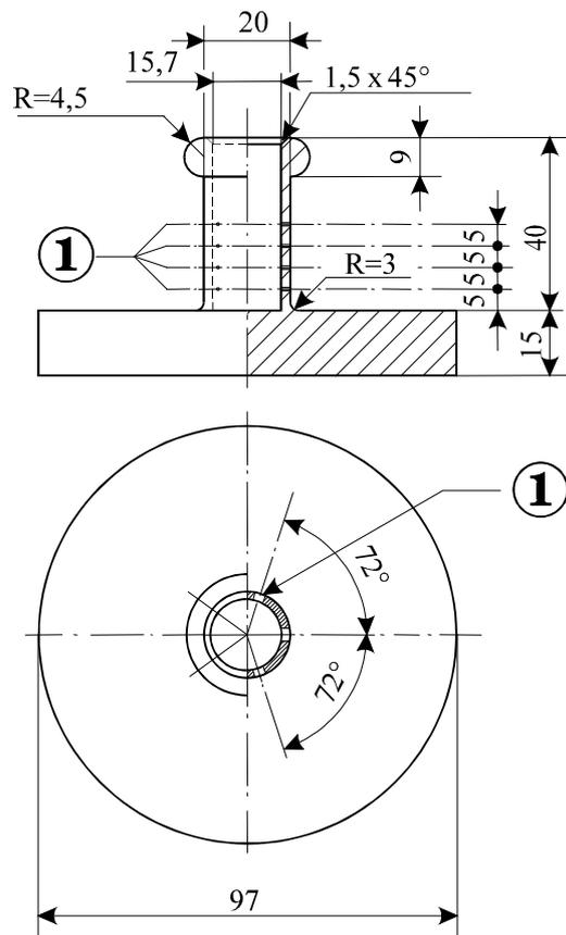
Fig. 3: Hollow bronze cylinder, closed at one end
