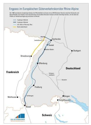
The contractually agreed extension of the Rhine Valley railway as an element of the NRLA concept is progressing slowly. The upgrade to four-track traffic, 740 metres train length and 2000 tonnes train weight is intended to significantly increase the line capacity and performance.
